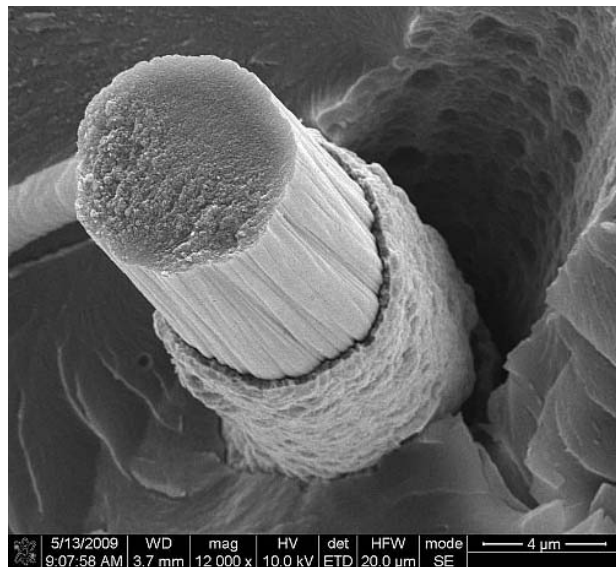
Nanofiber bundle coated with Ni, embedded in polymer substrate - applications in aeronautics (radar screening) - sample from INFN Rome
